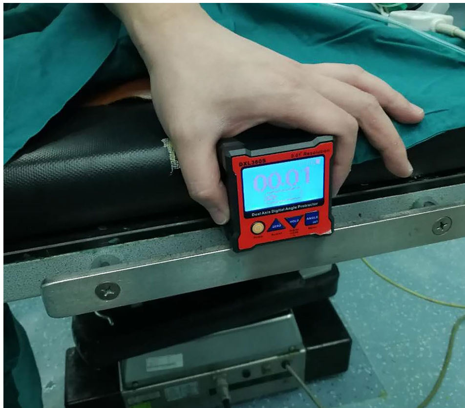
Fig. 1 The operating table is positioned horizontally to the floor
